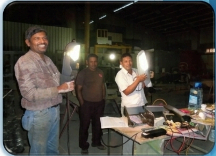
Testing LED Street Lights
